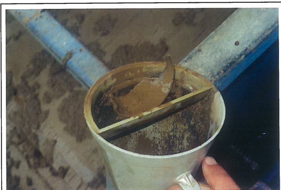
This piece of a cement float collar and additional cuttings were recovered after sweeping a well onshore South Louisiana drilled with a heavily weighted mud system.
