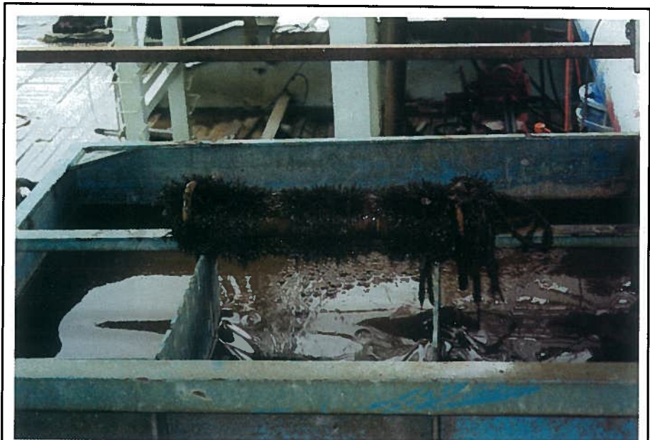
Metal fragments, slivers and burrs generated during milling operations become mated within synthetic fiber suspensions, greatly enhancing transport to the surface. Metal fragments recovered from a section milled at 11,200 feet in a well onshore Louisiana are shown here.
