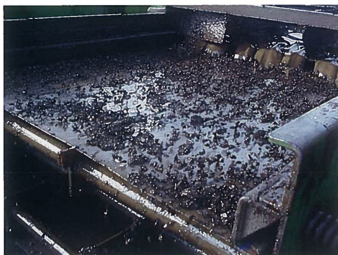
Figure 4. Fibre-impregnated solids screened and removed by solids control equipment.
