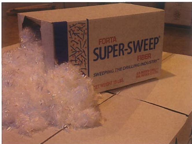
Figure 1. ½ in. long treated polypropylene fibre.
