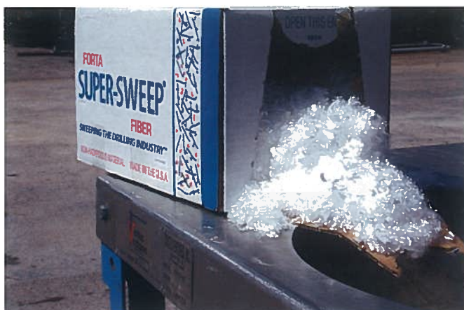
Figure 3. Fibre easily added at mud hopper.
