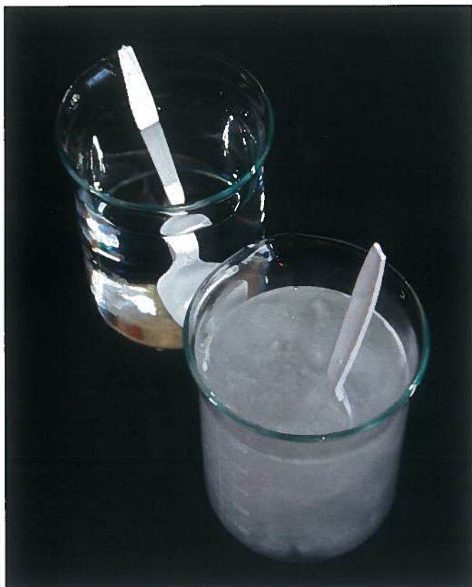
Figure 2. Fibre suspends without changing fluid viscosity.
